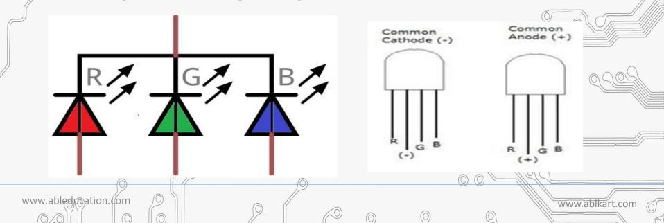
The one that we are going to use is the common anode RGB led. So, we will connect the common pin to the GND of Arduino and the other three leads of the led's to the digital pins of Arduino.
