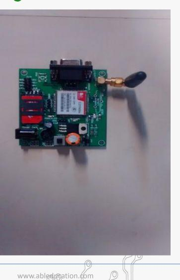
This is a very low cost and simple Arduino GSM and GPRS module. We use the module SIM Com SIM900A . It's the cheaper module now available In the market. This post will allow you to make arduino controlled calls and also send text messages.
