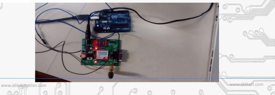
So we are supposed to use serial pins of Arduino (Rx and Tx). So if you are going with this method, you may connect the Tx pin of GSM module to Rx pin of Arduino and Rx pin of GSM module to Tx pin of Arduino.
